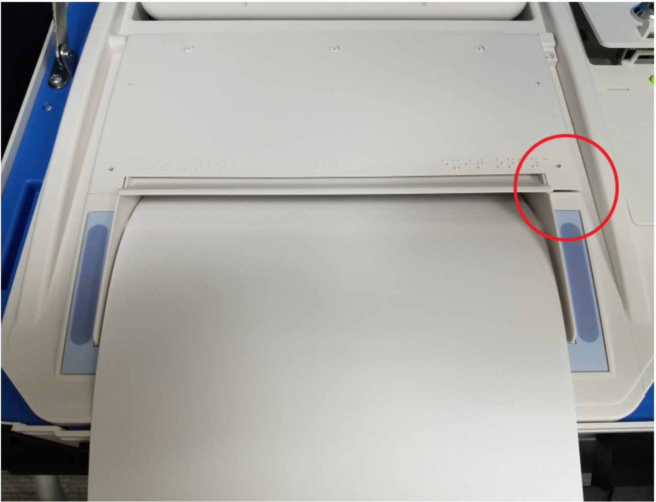
Figure 1: Touch Writer Duo Paper Feed Mechanical Issue
